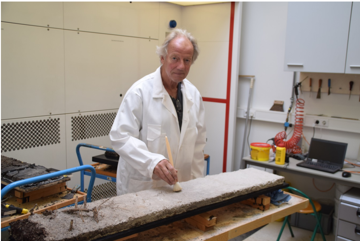
Figure 3. Testing new water-borne impregnants in the ISRIC workshop.
