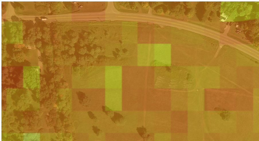
Figure 23. Ground overlay from PSP in the Chenango gravelly loam map unit, silt % 0–5 cm. Centre of image -76^{\circ}17'03'' E, 42^{\circ}22'40'' N
