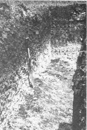
Trench about 10 m long to study small-scale lateral differences in a Typic Pellustert (Vertisol) with marked contrast between the dark solum and the underlying calcareous materials. The spade is 105 cm long.
