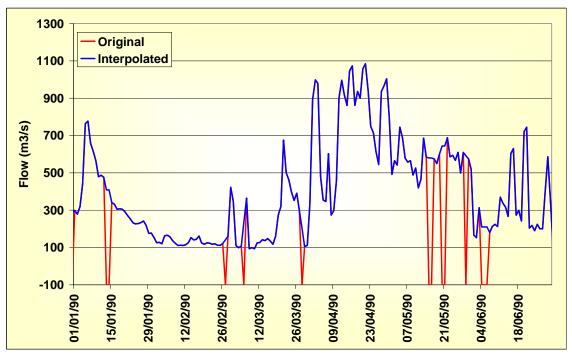
Figure 34: Examples of the interpolation of flow data
