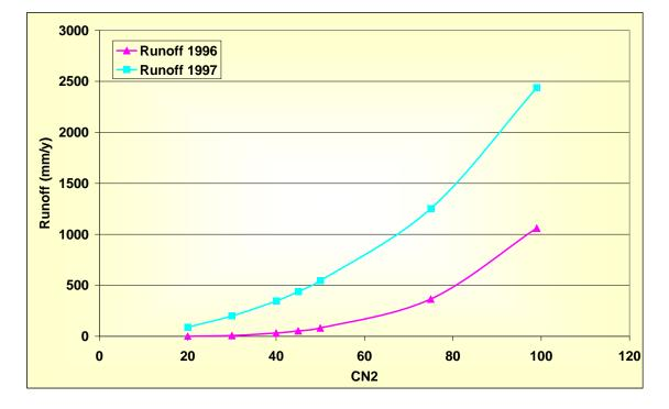
It is evident that a proper determination of the SCS curve number CN2 is essential. Less sustainable land use and land management, refelected by higher CN2 values, will increase runoff and soil erosion substantially (Figure 68 and Figure 69).
