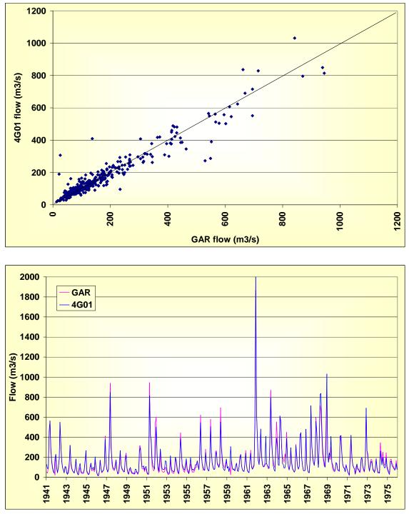
Figure 35: Comparison between data for Garissa from the Global Runoff Discharge Data (GAR) and from University of Nairobi (4G01)
