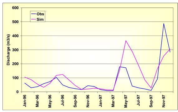
Figure 44: Observed and simulated inflows in Masinga reservoir (MasIn)
