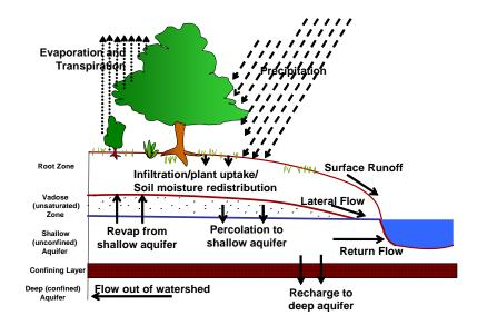
Figure 5: Main land-phase processes simulated within SWAT
