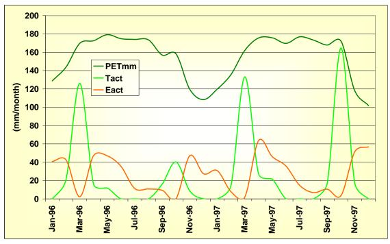
Figure 50: Potential and actual evapotranspiration under maize (HRU 686, subbasin 68)
