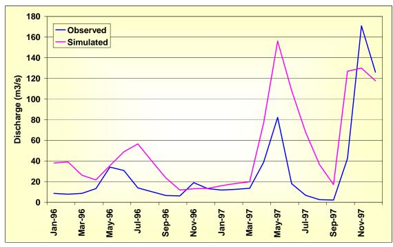
Figure 42: Observed and simulated flows of Thiba river (4DD01)
