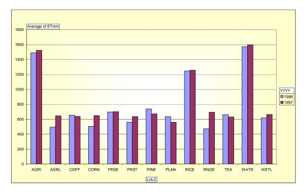
Figure 58: Mean actual evapotranspiration for the land classes defined for a dry year (1996) and a wet year (1997)
