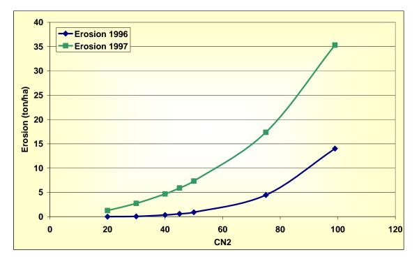
Figure 69: Sensitivity analysis of the curve number CN2 runoff coefficient for HRU 501 (tea) on erosion
