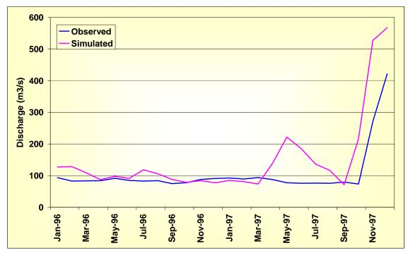
Figure 45: Observed and simulated inflows in Kiambere reservoir (KiaIn)
