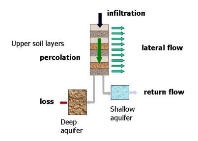
Figure 6: Sub-surface water fluxes simulated in SWAT
