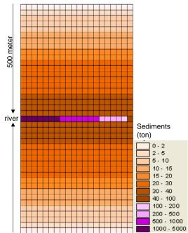
Figure 77: Projected erosion without green water management
