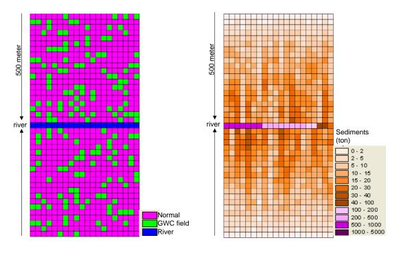
Figure 78: Projected erosion with random 20% uptake of green water management
