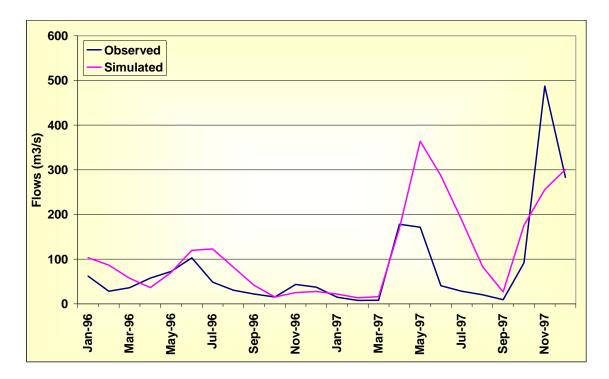
Figure 62: Comparison between observed and simulated inflow into Masinga reservoir
