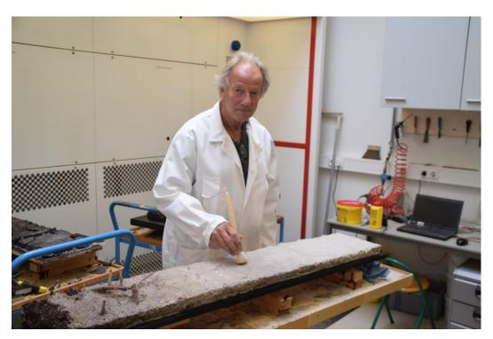
Figure 3. Testing new water-borne impregnants in the ISRIC workshop.
